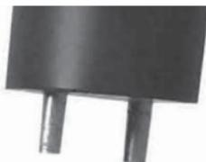
In order to work properly, the 2 measuring electrodes of the EC probe must be clean and in good condition (not broken or bent).
