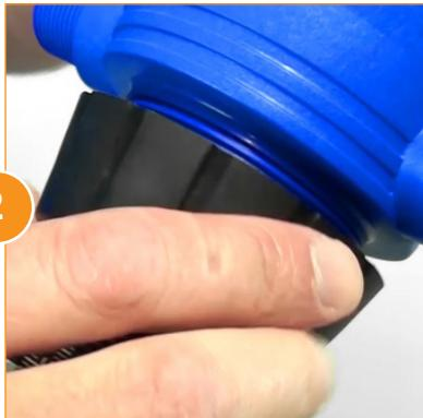
Unscrew the injection stem nut.
