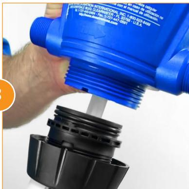
Pull the injection stem straight out from the body of the injector. Set the body aside.
