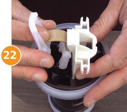
Now to insert both the valve support frame and the push rod into the piston shell, use your index finger to push on the spring. This will set everything into place and you will hear a click. If the parts aren't fitting together, just lift both subassemblies out and try again.
