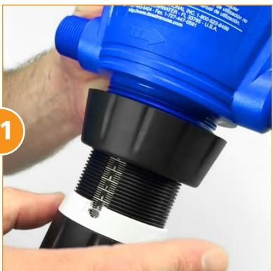
If the scale you prefer is not facing out, just loosen the stem nut and remove.
