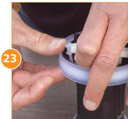
Insert the upper valves into the bottom of the upper area, snapping them into the valve support frame.
