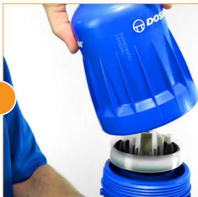
Begin by removing the piston from your Dosatron injector. Unscrew and remove the bell housing (you may use a universal strap wrench), pulling the piston out of the body. Set the bell housing and body aside.
