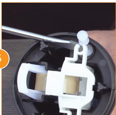
To remove the motor and valve support assembly from the piston shell, you will need a flat head screwdriver. Using the screwdriver, remove the upper valves from the guide. The valves look like golf tees and will drop down and out of the piston shell. Set them aside.
