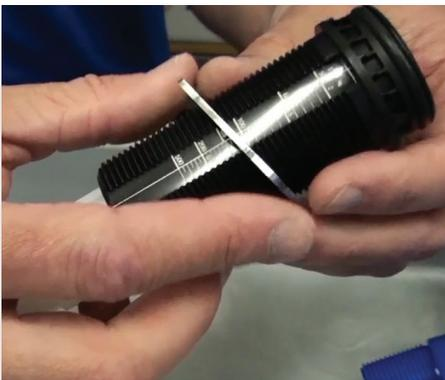
**Step 11:** Then, remove the metal retainer by sliding it straight down.
