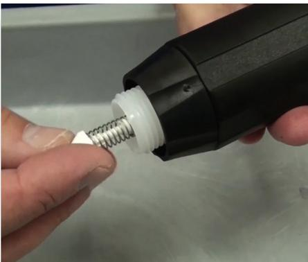
**Step 20:** Now, you can install the new check valve assembly into the stem.
