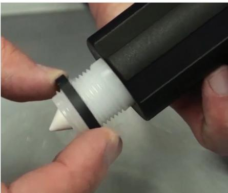
**Step 8:** Slide the anti-lock ring down and remove.
