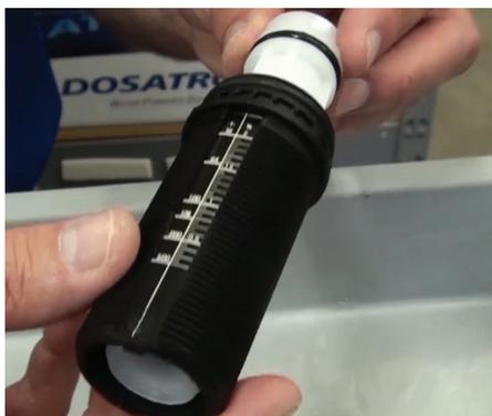
**Step 15:** Next, align the groove in the new white stem with the tooth inside the lower portion of the black sleeve and slide the stem down as far as possible.
