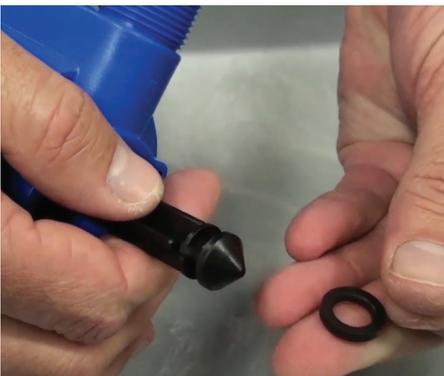
**Step 24:** Install the new seal into the groove on the plunger.
