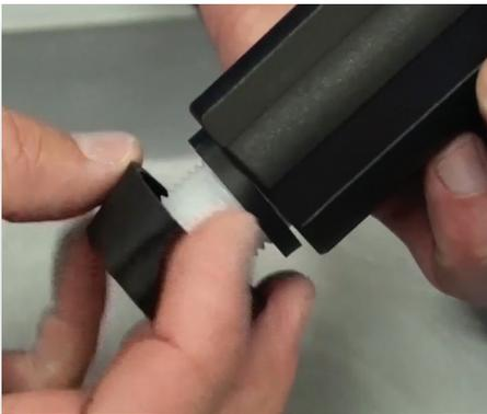
**Step 7:** Unscrew the lock nut
