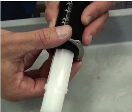
**Step 16:** Slide the metal retainer to the top of the black sleeve.
