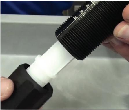
**Step 10:** Unscrew and remove the adjusting nut.
