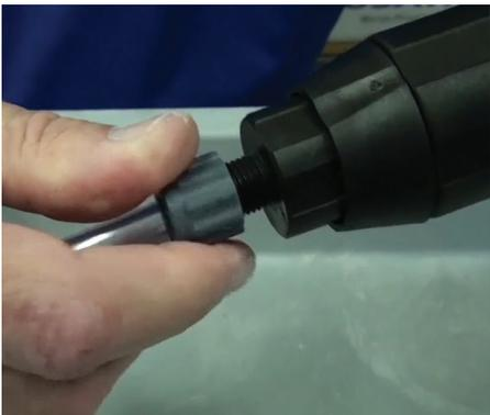
**Step 32:** Hand tighten the nut.
