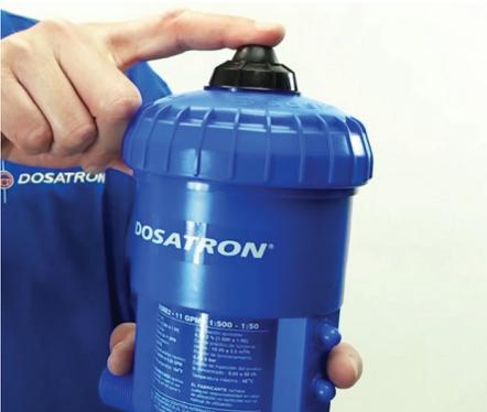
**Step 6:** If you don't see liquid moving up the tube or you don't feel suction on your finger, turn the water off. Press the air bleed button on the lid a couple times to release the pressure.
