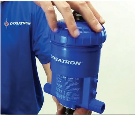
**Step 22:** Hand tighten the lid. The Injector should now be clicking and drawing concentrate.
