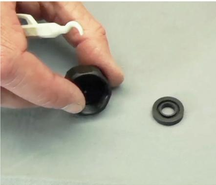
**Step 4:** Remove the check valve seal.
