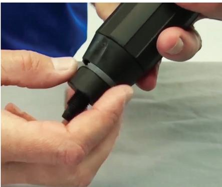
**Step 3:** Unscrew and remove the check valve barb (Part #:J051).
