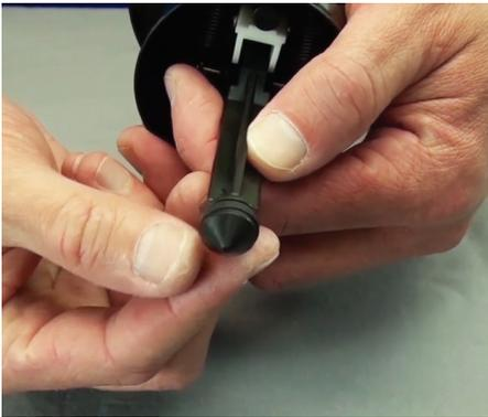
**Step 10:** Take a close look at the plunger seal for nicks, scratches, or wear. If you see damage or don't remember the last time you changed the seal, just replace it now.
