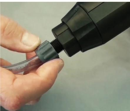
**Step 12:** Hand tighten the nut. This should stop the water from dripping back into the stock tank.
