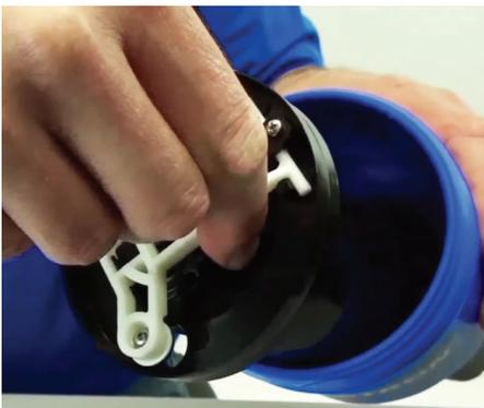
**Step 3:** Grasp the white valve support and pull the piston straight out of the body.
