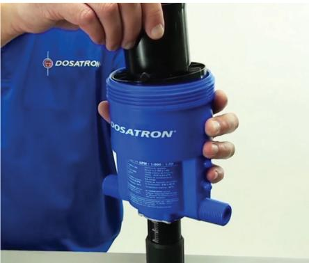
**Step 8:** Also, check the piston shell's fit inside the body. To do this, invert the piston and slide it into the body. It should be a snug fit. If it feels loose, the piston shell (Part #: P421) and the push rod o-ring (Part #: J020) need to be replaced.
