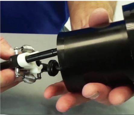
**Step 13:** Pull the actuator assembly out and discard the old piston shell.
