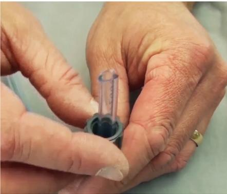
**Step 10:** Thread the suction hose nut onto the hose.
