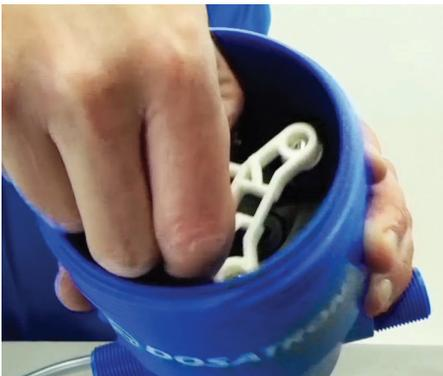
**Step 9:** Grasp the white valve support and pull the piston straight out of the body. Set the body aside.
