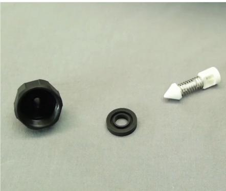
**Step 6:** Inspect the seal (Part #: J051) and the check valve assembly (Part #: MPDI122). If they are dirty, you may be able to soak, brush off, and reinstall. If you see damage or if you don't remember the last time you changed these parts, just replace them now.
