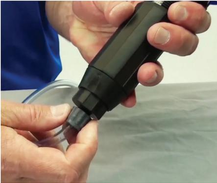
If your Injector is pushing water down into the concentrate container, it's time to investigate the check valve.
