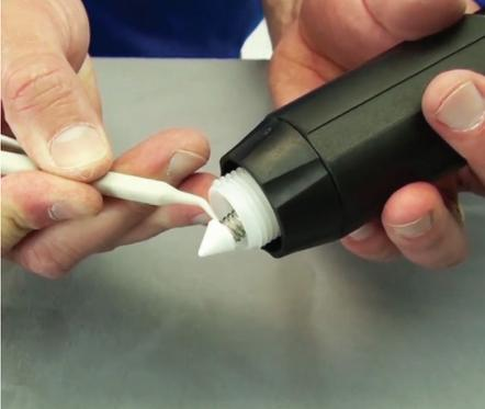
**Step 5:** Then carefully pry the check valve assembly down and out of the stem. A small flat blade screwdriver or pick (Part #: TOOL02) will make this easier.
