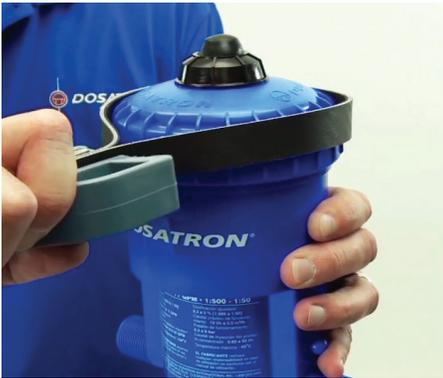
**Step 1:** If the unit isn't clicking, use a strap wrench (Part #: TOOL01) to loosen the lid.
