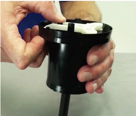
**Step 20:** Test the piston, by pressing the pushrod from the top and bottom, it should click each time.
