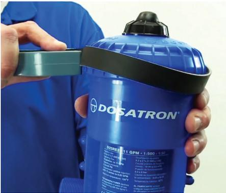
**Step 7:** Using a strap wrench (Part #: TOOL01), loosen the lid.
