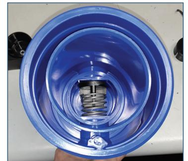
4. On the outlet side of the unit, unscrew the internal screw securing the bypass retainer.
