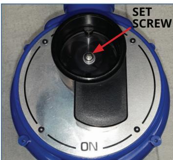
14. Install the black cap on top of the bypass knob in the proper position.
