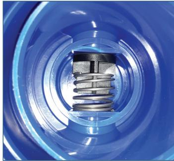
12. Install the bypass retainer as shown in the photo and secure the set screw.
