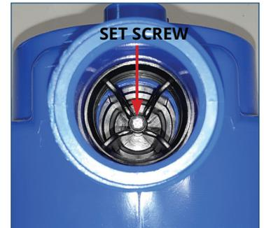
13. Back on the the top of the unit, install the bypass knob, as shown, and secure the set screw.
