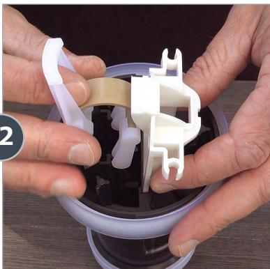
Now to insert both the valve support frame and the push rod into the piston shell, use your index finger to push on the spring. This will set everything into place and you will hear a click. If the parts aren't fitting together, just lift both subassemblies out and try again.
