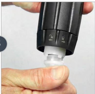
Grab the barb and pull the check valve assembly straight out. It usually comes out in two pieces. Discard all check valve parts.
