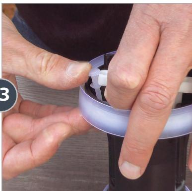
Insert the upper valves into the bottom of the upper area, snapping them into the valve support frame.
