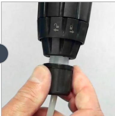
Unscrew the suction hose nut and remove the suction hose.
