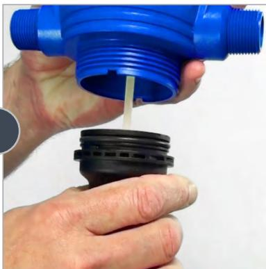
Pull the injection stem straight out from the body of the injector. Set the nut and body aside.
