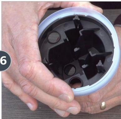
Align the tooth with the shell and press down and twist a quarter turn clockwise to lock. If it is difficult to twist or if the flange lifts up easily, just remove the flange, realign and try again.
