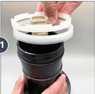
Slide the lock ring and Lower Flange up and off the black piston shell.
