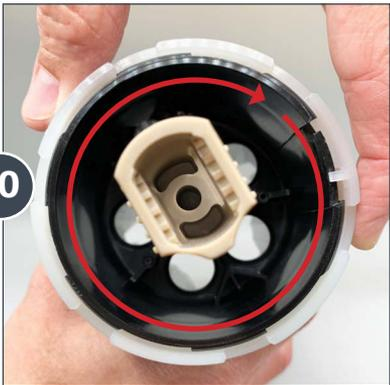
Rotate the lock ring about  $\frac{1}{2}$  of an inch clockwise to unlock, making sure the white tooth slides on top of the lever.
