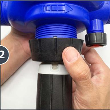
Reinstall the injection stem nut hand tight.
