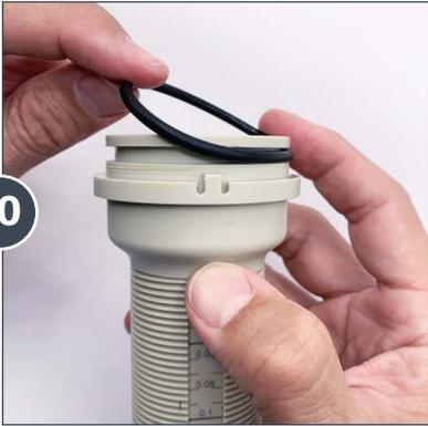
Remove and replace the **Injection Sleeve O-Ring (Part #: JDI100)**.
