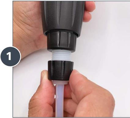
Unscrew the suction hose nut and remove the suction hose and ferrule from the bottom of the Dosatron unit.
