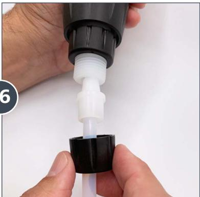
Slide the hose and ferrule onto the barb at the bottom of the Dosatron unit, then tighten the hose nut.
