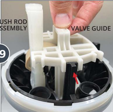
Align the valve rack next to the push rod assembly making sure the guide aligns with the black posts on the piston shell, and the lower valves align with the 4 center openings.
