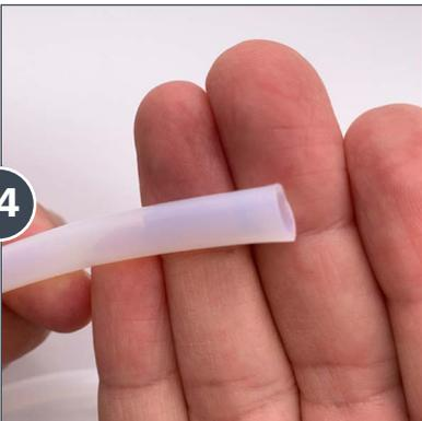
Before installing the suction hose, inspect it. If it flares out, cut an inch or so off and reinstall.
