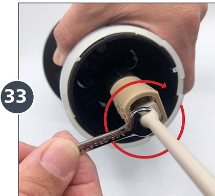
Insert the plunger back into the piston and with the use of the 8mm wrench, rotate it a quarter of a turn clockwise to lock it into place.
