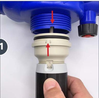
Carefully insert the plunger inside the top of the stem in a vertical motion to avoid bending the plunger.
