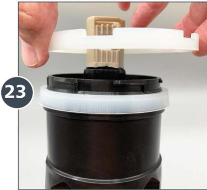
Hold the white lock ring with the flat edge facing down towards the piston, and place the lock ring on top of the **NEW Lower Flange**.
