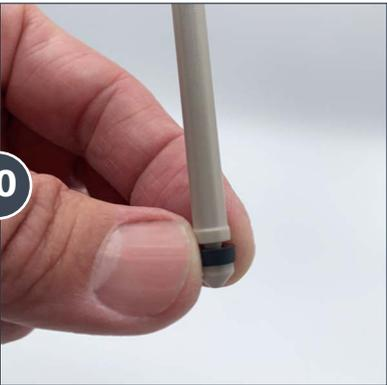
Set the stem aside and pick up the blue body. Remove and replace the **Plunger Seal (Part #: JDI200)**, by pinching it and rolling out of the plunger or using a small flat blade screwdriver.
