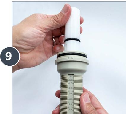
Push the white injection stem up and out of the graduated injection sleeve.
