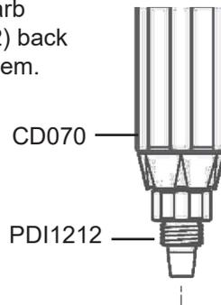
7. Rub a small amount of **Dosa-Lube** onto the injection sleeve o-ring (J024), and attach the injection stem assembly (CD070) back to the unit.
