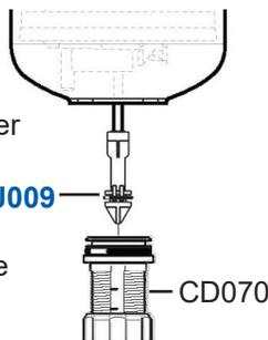
4. From the injection stem (CD070), unscrew the check valve barb (PDI1212) to remove the check valve assembly.
