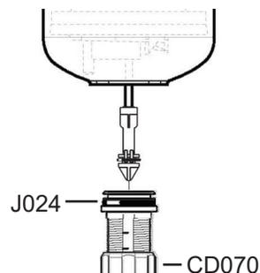
8. Reattach the injection stem assembly (CD070) to the unit by screwing the 4 screws (M337) back onto the silver plate (M079).
