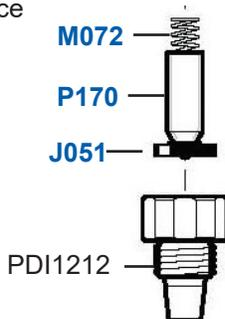
6. Insert the check valve assembly back into the injection stem (CD070). Screw the check valve barb (PDI1212) back to the stem.
