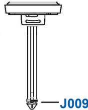
3. Hold the injection stem assembly and unscrew the check valve nut (PDI734). Pull out the check valve assembly (PJDI115).
