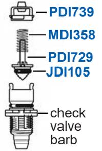
6. Apply **Dosa-Lube** on the check valve barb o-ring. Insert the updated check valve assembly (PJDI115) back into the bottom of the injection stem assembly (CDDI074), making sure the 4 keys on the check valve seat next to the 4 keys on the bottom of the stem. Screw the check valve nut (PDI734) back on.
