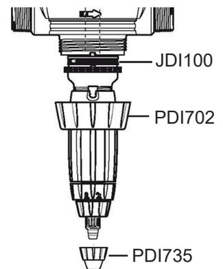
Cut 1" from the tip of the hose in a straight line. Insert the hose back onto the bottom of the check valve barb. Screw hose nut (PDI735) back on.
