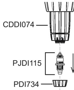
4. Give the top guide (PDI739) 1/4 of a turn counter clockwise to remove, and discard.
