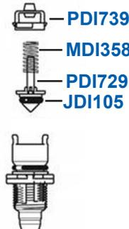
Discard the check valve spring (MDI358), check valve cone (PDI729) and check valve cone o-ring (JDI105).
