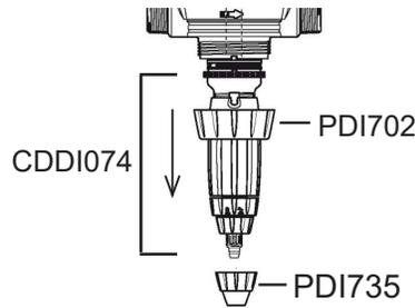
2. From the tip of the exposed plunger, remove the plunger seal (J009). Pinch the seal, roll it off, then replace with the new one.
