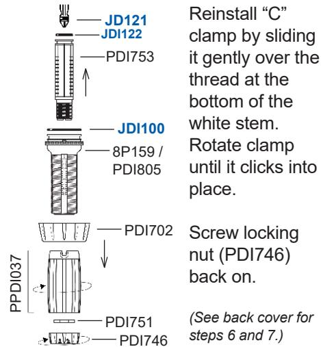
Reinstall "C" clamp by sliding it gently over the thread at the bottom of the white stem. Rotate clamp until it clicks into place.
