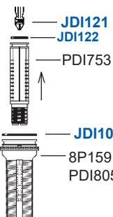
**!** To remove o-ring easily without tools, squeeze it on either side to raise the seal, then slide it over the groove
