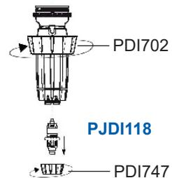
7. Push complete injection stem assembly in position at the bottom of the blue body, making sure desired scale is facing front of injector. Keys at the top of the black sleeve should slide into the slots at the bottom of the body. Slide injection stem nut (PDI702) up the sleeve and screw back on. Insert hose back onto the bottom of the check valve barb (**PJDI118**). Screw hose nut (PDI803) back on.
