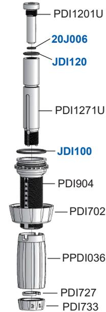
Reinstall "C" clamp by sliding it gently over the thread at the bottom of the white stem. Rotate clamp until it clicks into place. Screw locking nut (PDI733) back on.
