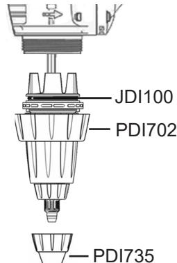
Cut 1" from the tip of the hose in a straight line. Insert the hose back onto the bottom of the check valve barb. Screw hose nut (PDI735) back on.
