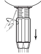
2. Remove old plunger seal (J029) with new one from kit.
