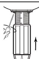
11. Unscrew inlet/outlet adapters (P252). Remove old black adapter seals (J534EP) and replace with new ones from kit. Screw inlet/outlet adapters (P252) back on.
