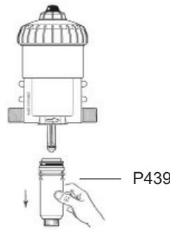
5. Insert the new check valve assembly (**MPDI122**) into the injection stem (P439) with the cone pointing out. Push the new check valve assembly as far as possible into the stem. Replace the check valve seal (**J051**) into the check valve barb (**P169**) with the groove facing up. Hand tighten the new check valve barb (**P169**) onto the injection stem (P439).
