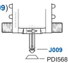
4. Unscrew the check valve barb (**P169**). Remove the check valve seal (**J051**). If the seal isn't visible at the end of the injection stem (P439), look inside the check valve barb (**P169**). Carefully pry the check valve assembly (**MPDI122**) out of the injection stem (P439) watching out not to damage the lower end of the injection stem. Replace injection sleeve o-ring (**J024**).
