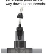
Hand tighten the nut onto the top of the injection stem.
