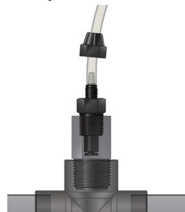
**8** Hand tighten the nut onto the top of the injection stem.
