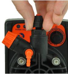
**2** Insert the rigid opaque tubing through the nut.
