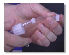
**Step 3:** Remove the nozzle, collar, and tube nut from the PVC suction tubing and set aside.
