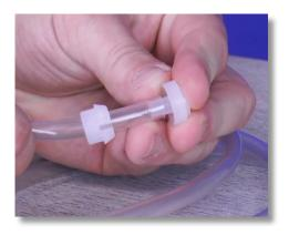
**Step 9:** Slide the collar back onto the tube. Make sure the collar's crown is pointed away from the tube nut. Then, insert the nozzle back onto the end of the tube's opening.
