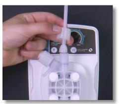
**Step 5:** Now locate the discharge valve tube nut. Unscrew the discharge valve tube nut and disconnect the tubing from the discharge valve.
