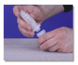
**Step 14:** If not, separate the foot filter into three (3) pieces by popping the filter basket from the filter body.
