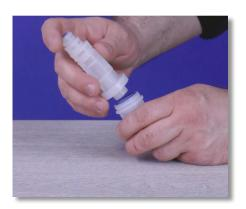
**Step 23:** Insert the filter basket into the filter body and forcefully pop them together.
