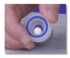
**Step 16:** Set the filter body aside and locate the ceramic ball in the filter seat.
