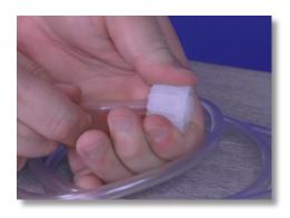
**Step 10:** Push the collar and nozzle together as close as possible, and pull the tube nut toward the nozzle to compress the collar and nozzle tight together, forming a ferrule connection.
