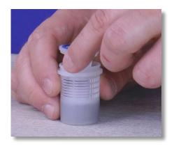
**Step 22:** Set the filter body down, grab the filter basket and put the filter seat back into the filter basket.
