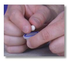
**Step 20:** Put the ceramic ball back into the filter seat and set the filter seat aside.
