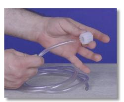
**Step 8:** Grab the suction valve tube nut and slide one end of the flexible PVC suction tubing through the outside opening of the tube nut.
