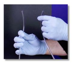
**Step 6:** Visually inspect the condition of the PVC suction tubing. Look at both ends of the tube, if either end is flared, use the diagonal pliers to cut the flared portion off. If the tubing is cracked, old, or broken, you need to replace it now.
