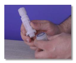
**Step 15:** The filter seat may stick to the filter body. Make sure the filter seat rests in the filter basket instead, to avoid losing the ceramic ball.
