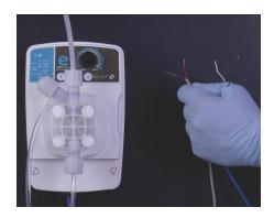
**Step 5:** If the connection is fine, dis-connect the water meter and the **eMP** lead wires from each other.
