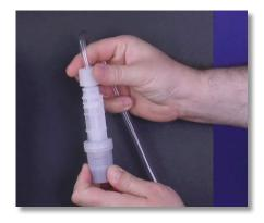
**Part 5b** - If the alarm LED on the **eMP** is Green, inspect the suction tubing, tubing connections, and foot filter.
