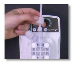
**Step 16:** Reattach the tube onto the discharge valve by hand tightening the tube nut. Do not cross thread nor overtighten.
