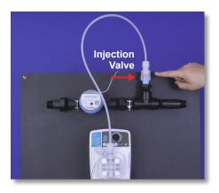
**Part 6b:** If the alarm LED on the **eMP** is Red, inspect the discharge tubing, tubing connections, and injection valve.
