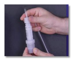
**Step 25:** Grab the PVC suction tubing and connections hanging from the suction valve of the pump. Reattach the tubing connections to the foot filter by hand tightening the tube nut. Do not cross thread or overtighten.
