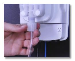
**Step 11:** Reattach the tube and tubing connections onto the suction valve of the pump head by hand tightening the tube nut. Do not cross thread or overtighten.
