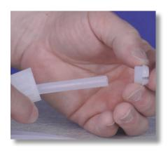
**Step 10:** Grab the polyethylene discharge tubing and the injection valve connections you set aside earlier.
