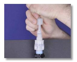
**Step 3:** Unscrew the tube nut from the injection valve.
