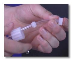
**Step 5:** Remove the nozzle, collar, and tube nut from the PVC suction tube, and set aside.
