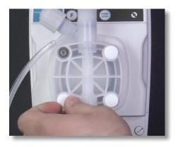
**Step 30:** Reinsert the four (4) white screw caps back over the pump head screws.
