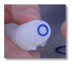
**Step 21:** Grab the filter body and inspect to make sure the small blue o-ring on top of the filter body is not damaged.
