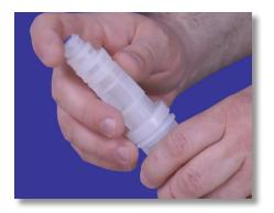
**Step 24:** Pull on the two (2) sections to make sure they are connected securely and shake the foot filter back and forth once more, verifying the ceramic ball is moving freely.
