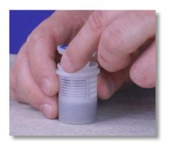
**Step 17:** Pull the filter seat out of the filter basket and set the filter basket aside.
