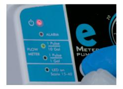
**Step 7:** Switch programs by putting the pump in **Standby Mode** and press the '**F**' or Function button. If the **eMP** works by itself, it is time to test the water meter.
