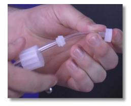
**Step 12:** Reattach the foot filter tubing connections onto the loose end of the tube. Be mindful of their orientation. Push the collar and nozzle together as close as possible. Pull the tube nut toward the nozzle to compress the collar and nozzle tight together, forming a ferrule connection.
