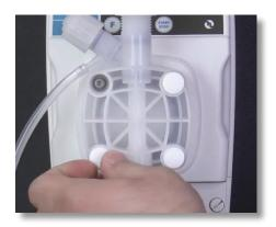
**Part 5c -** If the alarm LED on the **eMP** is Green, tighten the pump head.
