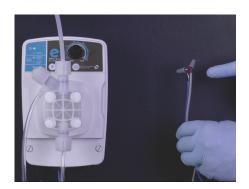
**Step 4:** If the issue persists, inspect the connection of the water meter to the **eMP** to see if it is loose, or has been disconnected.
