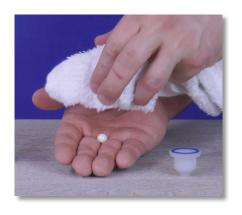
**Step 18:** Pour the ceramic ball out of the filter seat and into your hand. Set the filter seat down and use the small towel to wipe the ceramic ball clean. Do not misplace it.
