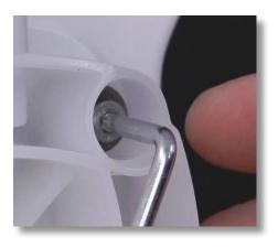
**Step 29:** Using the 3mm Allen wrench, tighten the four (4) pump head screws about 1/8 turn each. It's best to tighten in a crisscross pattern.
