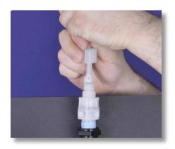
**Step 13:** Reattach the tube to the injection valve by hand tightening the tube nut. Do not cross thread nor overtighten.
