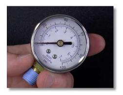
**Part 6a:** If the alarm LED on the **eMP** is Red, assess the pressure of the installation.
