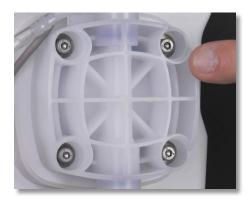
**Step 28:** Underneath the caps are four (4) pump head screws.
