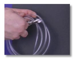
**Step 7:** Cut the PVC suction tubing so that the foot filter will comfortably sit in the chemical bucket in a vertical position from the suction valve. Set the remaining PVC tubing aside.
