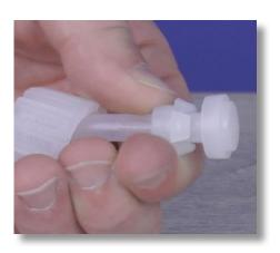
**Step 6:** Remove the connections, and set them aside. Visually inspect the condition of the rigid polyethylene discharge tubing.
