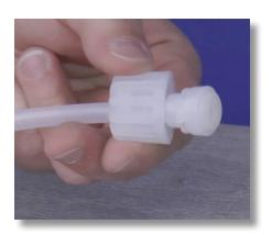
**Step 15:** Push the collar and nozzle together as close as possible. Pull the tube nut toward the nozzle to compress the collar and nozzle tight together, forming a ferrule connection.
