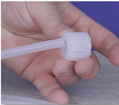
**Step 24:** Slide one end of the rigid polyethylene Discharge Tubing through the outside opening of the tube nut.
