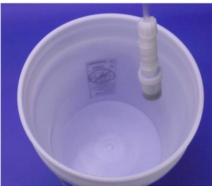
**Step 57:** Place the Foot Filter into the bucket or stock tank. This ensures the Foot Filter draws chemistry once you begin operation.
