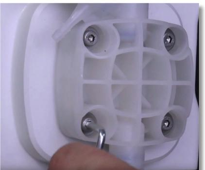
**Step 18:** Use the Allen wrench to carefully hand-tighten the four (4) Pump Head screws in a crisscross pattern until evenly snug.
