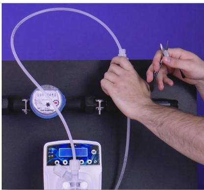
**Step 33:** Grab the rigid polyethylene Discharge Tube connected to the Discharge Valve. Using diagonal pliers or cutters, cut the tube so that it runs comfortably from the Discharge Valve to the Injection Valve.
