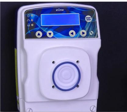
**Step 9:** If the blue o-ring is not there, still discard the Pump Head and connected items, but check to see if the blue o-ring is stuck to the **eOne MF** pump.
