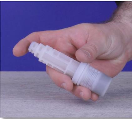
**Step 52:** Shake the Foot Filter back and forth once more, verifying the ceramic ball is moving freely. Set the Foot Filter aside.
