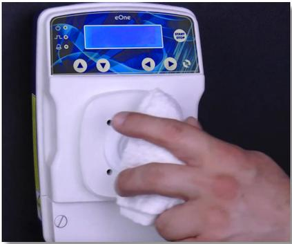
**Step 11:** Using the small towel, wipe clean the diaphragm and any other chemical stricken parts on the pump.
