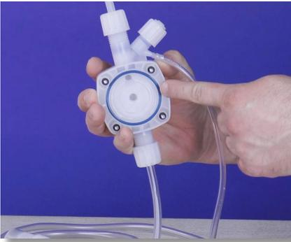
**Step 8:** Once removed, check the backside of the Pump Head to see if the blue o-ring is in the groove.
