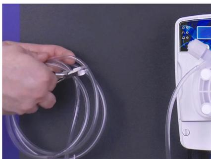
**Step 60:** Using the diagonal pliers, cut the tube so that it is long enough for the chemical bleed off to go into the bucket or stock tank while priming the **eOne MF** pump.
