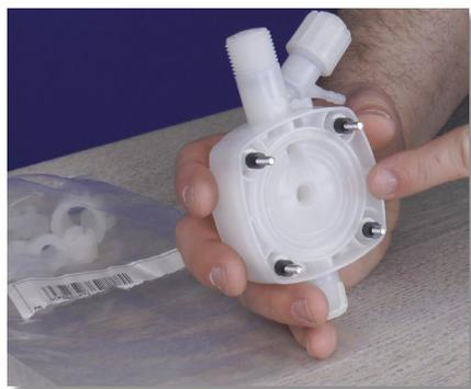
**Step 15:** Take the new Pump Head out of its bag, and turn it over so you are looking at the backside of the Pump Head.
