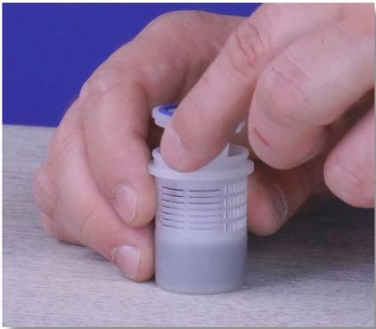
**Step 47:** Pull the filter seat out of the filter basket and set the filter basket aside.
