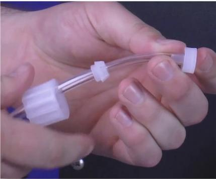
**Step 18:** Reattach the Foot Filter Tubing Connections onto the loose end of the tube. Be mindful of their orientation. Push the Collar and Nozzle together as close as possible. Pull the Tube Nut toward the Nozzle to compress the Collar and Nozzle tight together, forming a ferrule connection.
