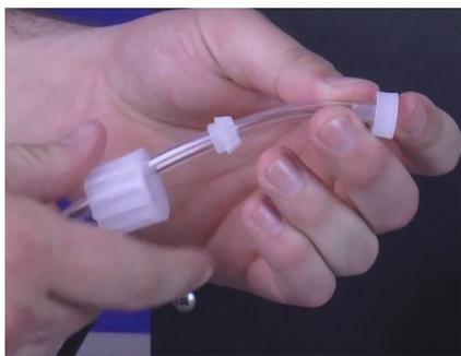
**Step 8:** Remove the Nozzle, Collar, and Tube Nut from the PVC Suction Tubing and set aside. Do not lose them.
