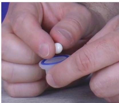
**Step 26:** Put the ceramic ball back into the filter seat and set the filter seat aside.
