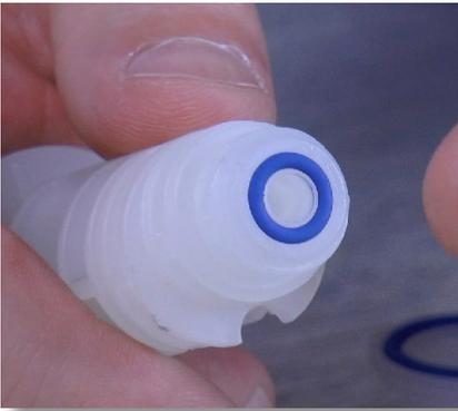
**Step 27:** Grab the filter body and inspect to make sure the small blue o-ring on top of the filter body is not damaged.
