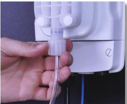
**Step 10:** Disconnect the Suction Valve Tubing Connections from the Pump Head by unscrewing the Suction Valve Tube Nut.
