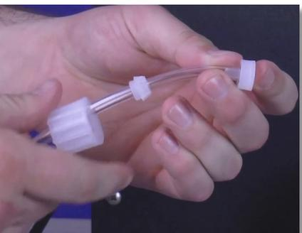
**Step 11:** Remove the Nozzle, Collar, and Tube Nut from the PVC Suction Tube and set aside. Do not lose them.
