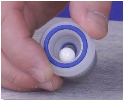
**Step 22:** Set the filter body aside and locate the ceramic ball in the filter seat.
