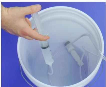
**Step 40:** Eject the chemistry from the syringe into the chemical bucket.
