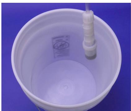
**Step 6:** Lift the PVC Suction Tubing, along with the Foot Filter out of the chemical bucket or stock tank.
