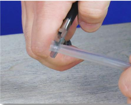
**Step 12:** Visually inspect the condition of the PVC Suction Tubing. If either end is flared, use the diagonal pliers to cut the flared portion off.
