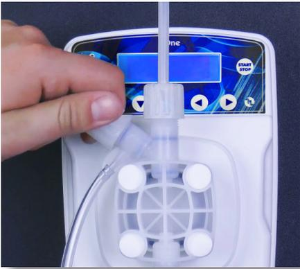
**Step 42:** Now close the Air Bleed Valve by turning it clockwise.
