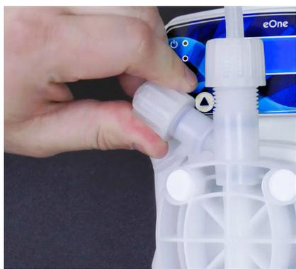
**Step 37:** Locate the Air Bleed Valve on the upper left portion of the Pump Head and open it by turning the valve counter-clockwise.
