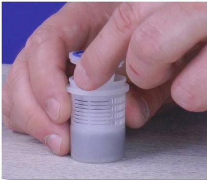
**Step 23:** Pull the filter seat out of the filter basket and set the filter basket aside.
