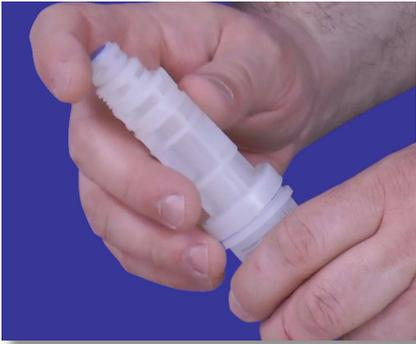
**Step 30:** Pull on the two (2) sections to make sure they are connected securely and shake the Foot Filter back and forth once more, verifying the ceramic ball is moving freely.
