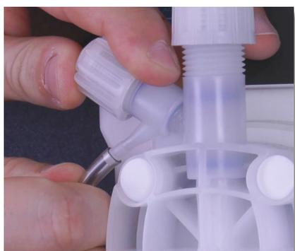
**Step 41:** Slide the bleed-off tubing back onto the Air Bleed Barb and place the tubing back into the chemical bucket.
