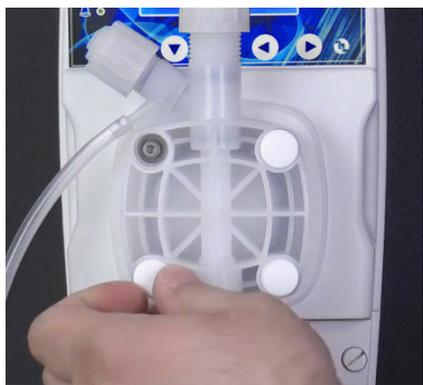
**Step 36:** Reinsert the four (4) white screw caps back over the Pump Head Screws.
