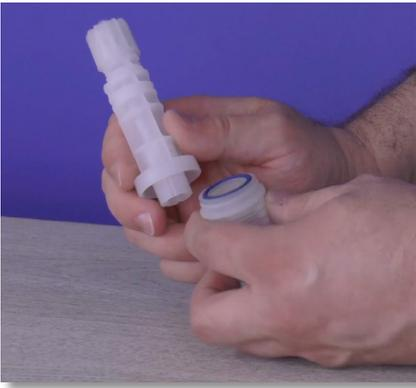
**Step 21:** The filter seat may stick to the filter body. Make sure the filter seat rests in the filter basket to avoid losing the ceramic ball.
