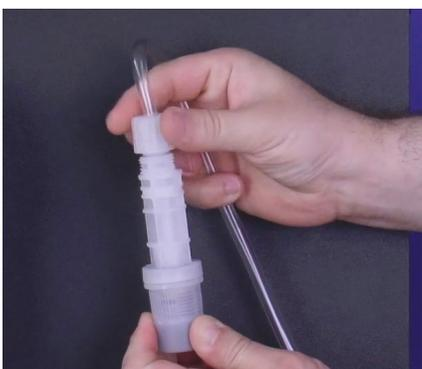
**Step 7:** Disconnect the Tubing Connections from the Foot Filter by unscrewing the Foot Filter Tube Nut.
