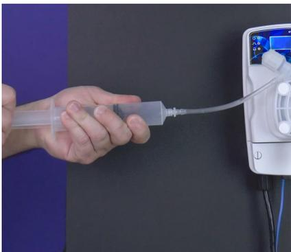
**Step 39:** Using the Syringe Kit, slide the 4mm adapter of the syringe onto the Air Bleed Barb and draw the plunger back. Chemistry should enter the syringe. This may take a couple of tries.
