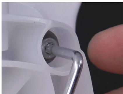
**Step 18:** Underneath the caps are four (4) Pump Head Screws. Using the 3mm Allen wrench, tighten the four (4) screws about 1/8 turn. It's best to tighten in a crisscross pattern.
