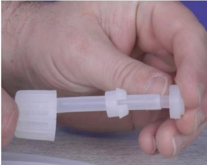
**Step 14:** Grab the Discharge Valve connections you set aside earlier and reattach the Tubing Connections back onto the loose end of the tube.
