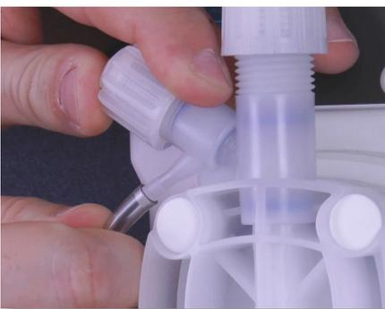
**Step 21:** Remove the bleed-off tubing from the Air Bleed Barb and set it outside of the chemical bucket.
