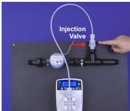
**Part 4b - If the pump draws chemistry but does not inject, inspect the Discharge Tubing, Tubing Connections, and Injection Valve:**
