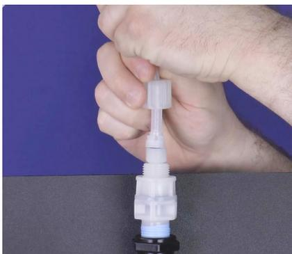
**Step 3:** Unscrew the Tube Nut from the Injection Valve. Be careful not to lose or misplace the blue Injection Valve O-Ring when removing the Tubing Connections.
