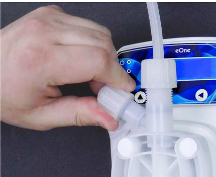
**Part 4d - If the pump draws chemistry but does not inject, release airlock from the Pump Head:**
