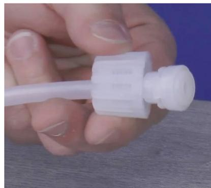
**Step 12:** Pull the Tube Nut toward the Nozzle to compress the Collar and Nozzle tight together, forming a ferrule connection.
