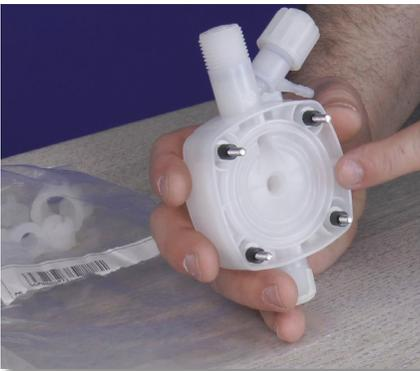
**Step 15:** Take the new Pump Head out of its bag, and turn it over so you are looking at the backside of the pump head.
