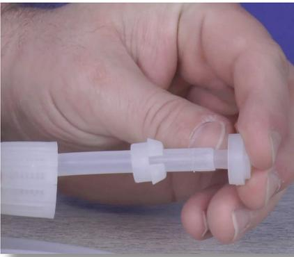
**Step 26:** Grab the nozzle and insert the pointed end into the opening of the same tube.
