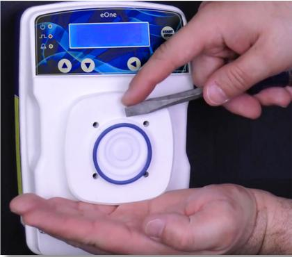
**Step 10:** If so, remove and discard the blue o-ring now. This can be done with your finger or flat blade screwdriver.
