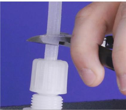
**Step 6:** Use the diagonal pliers or cutters to cut the tube as close to the old Injection Valve as possible.
