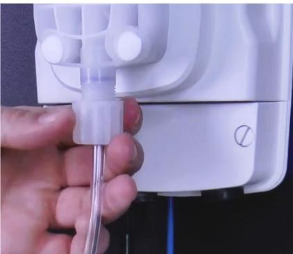
**Step 42:** Attach the tube, and tube connections onto the suction valve by hand tightening the tube nut. Do not cross thread nor overtighten.
