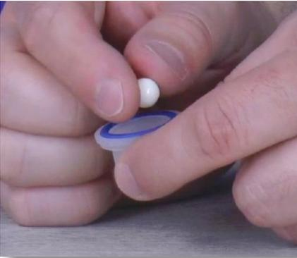
**Step 49:** Put the ceramic ball back into the filter seat.
