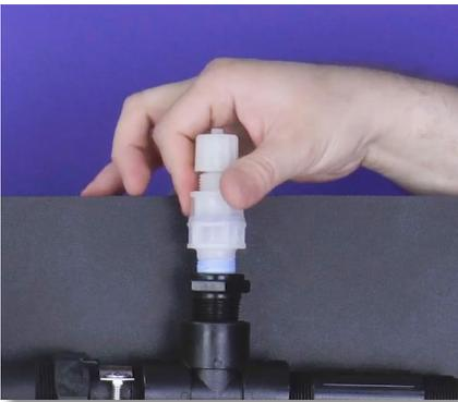
**Step 12:** Unscrew, disconnect, and discard the old Injection Valve from the installation saddle or tee.
