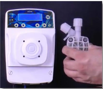
**Step 17:** To install the new Pump Head, align it so that the Y-shape points upward on the eOne pump.
