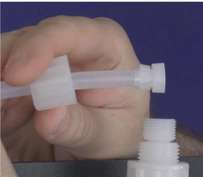
**Step 35:** Push the collar and nozzle together as close as possible.
