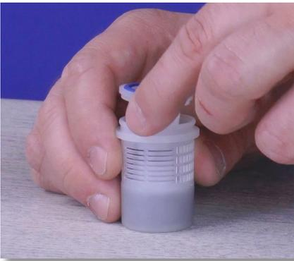
**Step 47:** Pull the filter seat out of the filter basket and set the filter basket aside.
