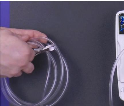
**Step 60:** Using the diagonal pliers, cut the tube so that it is long enough for the chemical bleed off to go into the bucket or stock tank while priming the **eOne** pump.
