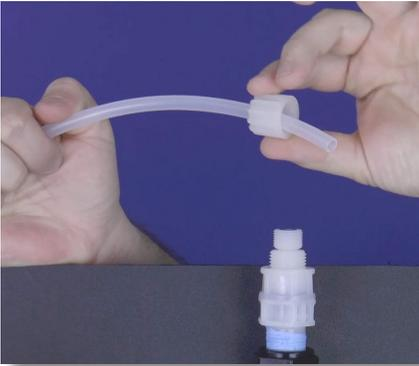
**Step 34:** Re-attach the tube connections onto the loose end of the connected Discharge tubing. Be mindful of their orientation for the tubing connections.
