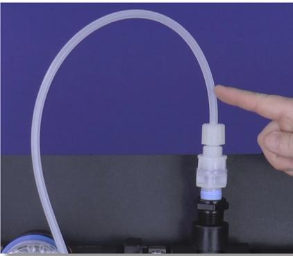
**Step 5:** Locate the used rigid Discharge tubing connected to the old Injection Valve.
