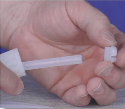
**Step 25:** Slide the collar onto the tube, and make sure the collar's crown is pointing away from the tube nut.
