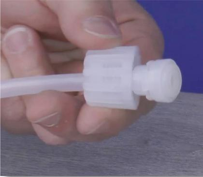
**Step 28:** Pull the tube nut toward the nozzle to compress the collar and nozzle tight together, forming a ferrule connection.
