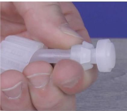
**Step 27:** Push the collar and nozzle together as close as possible.
