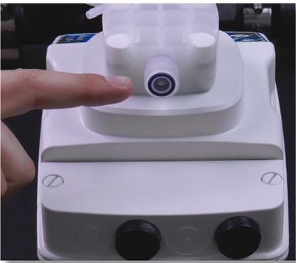
**Step 38:** Make sure you don't lose the blue o-ring directly at the bottom of the Suction Valve.
