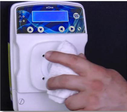
**Step 11:** Using the small towel, wipe clean the diaphragm and any other chemical stricken parts on the pump.
