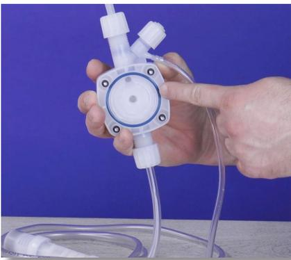
**Step 8:** Once removed, check the backside of the pump head to see if the blue o-ring is in the groove.
