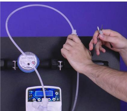
**Step 33:** Grab the rigid polyethylene Discharge tube connected to the Discharge Valve. Using diagonal pliers or cutters, cut the tube so that it runs comfortably from the discharge valve to the Injection Valve.
