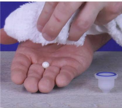
**Step 48:** Pour the ceramic ball out of the filter seat and into your hand and use the small towel to wipe the ceramic ball clean. Do not misplace it.
