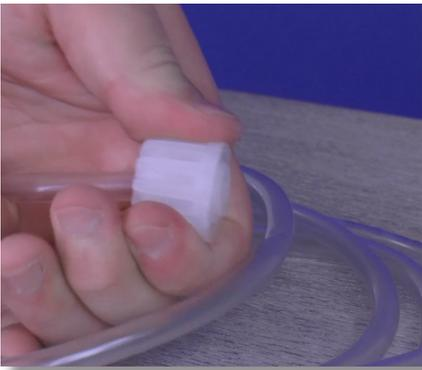
**Step 41:** Push the collar and nozzle together as close as possible. Pull the tube nut toward the nozzle to compress the collar and nozzle tight together, forming a ferrule connection.
